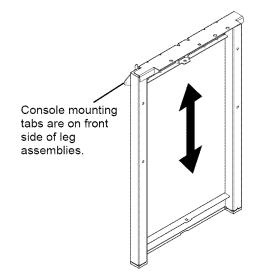
4. Insert non-locking casters into the caster plugs on rear of leg assembiles.
